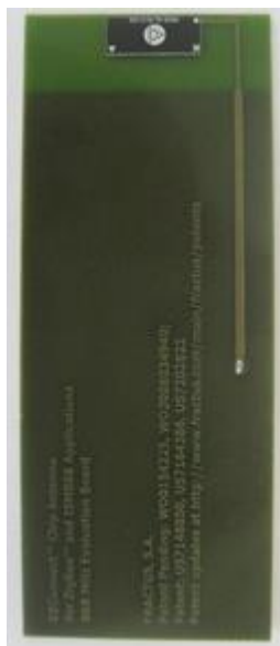
Figure 2 – Evaluation board at 868 MHz and graph of VSWR and Efficiency vs. Frequency (GHz)
