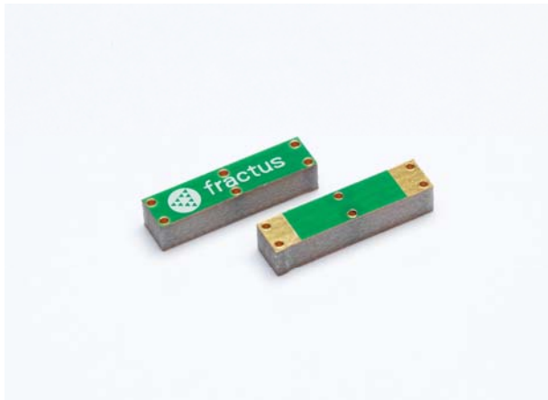
RUN mXTEND™ antenna component
