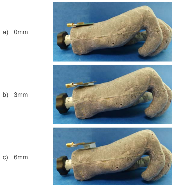
Figure 5 – Different distances between the phantom hand and the evaluation board that provide operation from 2.4GHz to 2.5GHz.
