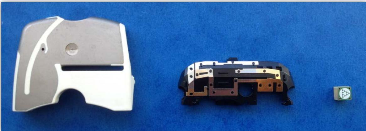
Fig. 4 Fifteen years of handset antenna evolution. A first dual-band internal antenna (left) obtained by grouping two antennas into a conjoined antenna set (year 1999); a state-of-the-art antenna (center) taking benefit of complexity to optimize the packaging of five frequency bands (year 2011); the mXTEND™ Antenna Booster replacing both (right) (year 2013).
