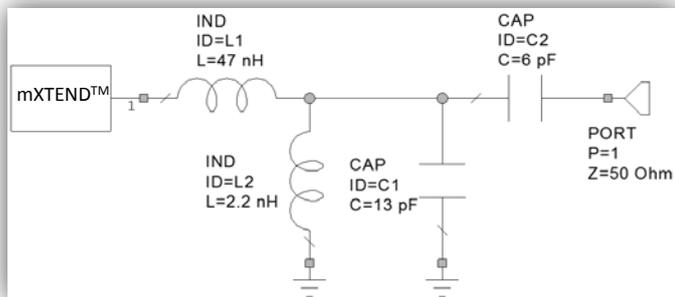
Fig. 7 Matching network designed to cover the low frequency region (824-960MHz). The components are SMD 0402 commercially available.
