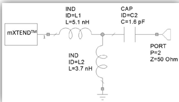
Fig. 8 Matching network for the high frequency region (1710-2690MHz). The components are SMD 0402 commercially available.
