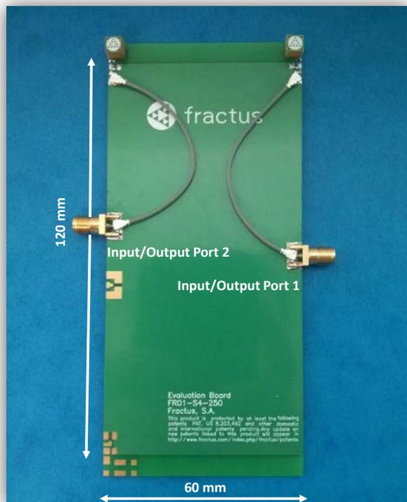
Fig. 6 Evaluation Board (Part Number: EB\_FR01-S4-250-UFL2R) integrating two mXTEND™ Antenna Boosters (Part Number: FR01-S4-250).
