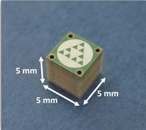
Fig. 5 Detailed view of the mXTEND™ Antenna Booster (Part Number: FR01-S4-250) emphasizing its reduced dimensions of just 125 mm<sup>3</sup>.
