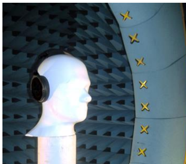
Antenna efficiency measurement of a headset in an anechoic chamber (3D pattern integration). Test includes a phantom head.
