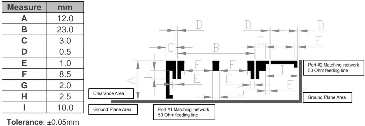
**Figure 8** – Footprint dimensions for the single chip antenna component.
